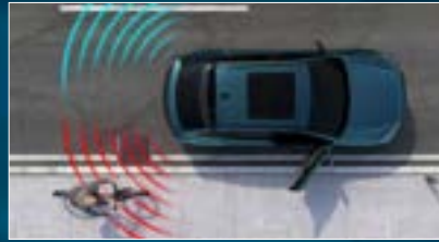
The Door Open Warning system helps prevent accidents while parked, by monitoring hazards around the vehicle.
