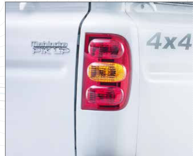
AUTOMATICALLY ACTIVATED HAZARD LIGHTS IN CASE OF SUDDEN BRAKING
