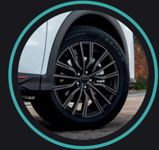
235/55R19 wheels with tyre pressure monitoring system
